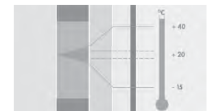
Air layer + insulation reduce difference in temperatures
