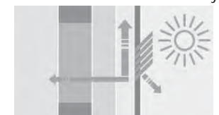
In summer, part of the heat is evacuated by circulating air
